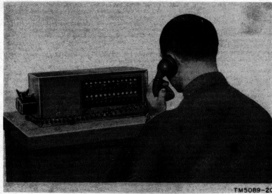
Figure 1. Intercommunication Station LS-202/FI, operational view.
